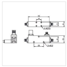
RF Solution offer a wide selection of Coupler for global customers. CP30-F1543-S-2-18GHz is a Coupler in Frequency Range of 2.0-18.0 GHz. It is made of high quality materials under a high standard, the Insertion Loss Max of this product is 0.7 dB, Nominal Coupling is  $30\pm1$  dB and Coupling Sensitivity is  $\pm1.0$  dB. The component has a good working performance and stability, it is ideal for handling a Rated Power of 50 W.
