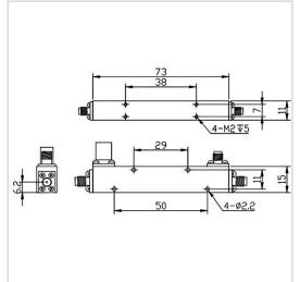
RF Solution offer a wide selection of Coupler for global customers. CP30-F1573-S-1-18GHz is a Coupler in Frequency Range of 1.0-18.0 GHz. It is made of high quality materials under a high standard, the Insertion Loss Max of this product is 1.2 dB, Nominal Coupling is  $30\pm1$  dB and Coupling Sensitivity is  $\pm1.0$  dB. The component has a good working performance and stability, it is ideal for handling a Rated Power of 50 W.
