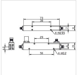
RF Solution offer a wide selection of Coupler for global customers. CP30-F1573-S-1-4GHz is a Coupler in Frequency Range of 1.0-4.0 GHz. It is made of high quality materials under a high standard, the Insertion Loss Max of this product is 0.5 dB, Nominal Coupling is  $30\pm1$  dB and Coupling Sensitivity is  $\pm0.7$  dB. The component has a good working performance and stability, it is ideal for handling a Rated Power of 50 W.
