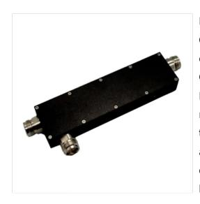
RF Solution offer a wide selection of Low PIM Couplers Combined or Open Circuit for global customers. CPXX-F4818-0.38-3.8 is a Low PIM Couplers Combined or Open Circuit in Frequency Range of  $0.38 \sim 3.8$  GHz. It is made of high quality materials under a high standard, the Coupling Loss of this product is  $\pm 1.2$  dB, Insertion Loss Max is 2.3 dB and Isolation Min is 23 dB. The component has a good working performance and stability, it is ideal for handling a Rated Power of 300 W.
