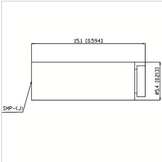
RF Solution offer a wide selection of Coaxial Fixed Termination (Dummy Load) for global customers. CT-02W-RA0515-SMPJ-40G is a Coaxial Fixed Termination (Dummy Load) in Frequency Range of DC~40.0 GHz. It is made of high quality materials under a high standard, the Connector Type of this product is SMP-M (J), VSWR Max is 1.30 and Impedance is 50  $\Omega$ . The component has a good working performance and stability, it is ideal for handling a Power of 2 W.
