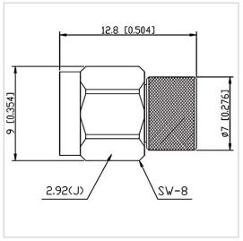
RF Solution offer a wide selection of Coaxial Fixed Termination (Dummy Load) for global customers. CT-02W-RA0713-2.92J-40G is a Coaxial Fixed Termination (Dummy Load) in Frequency Range of DC~40.0 GHz. It is made of high quality materials under a high standard, the Connector Type of this product is 2.92-M (J), VSWR Max is 1.20 and Impedance is 50  $\Omega$ . The component has a good working performance and stability, it is ideal for handling a Power of 2 W.
