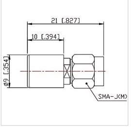
RF Solution offer a wide selection of Coaxial Fixed Termination (Dummy Load) for global customers. CT-02W-RA0910-SJ-12.4G is а Coaxial Termination (Dummy Load) in Frequency Range of DC~12.4 GHz. It is made of high quality materials under a high standard, the Connector Type of this product is SMA-M (J), VSWR Max is 1.25 and SMA-J(M) Impedance is 50  $\Omega$ . The component has a good working performance and stability, it is ideal for handling a Power of 2 W.
