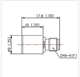
RF Solution offer a wide selection of Coaxial Fixed Termination (Dummy Load) for global customers. CT-02W-RA0910-SK-12.4G is a Coaxial Fixed Termination (Dummy Load) in Frequency Range of DC~12.4 GHz. It is made of high quality materials under a high standard, the Connector Type of this product is SMA-F (K), VSWR Max is 1.25 and Impedance is 50  $\Omega$ . The component has a good working performance and stability, it is ideal for handling a Power of 2 W.
