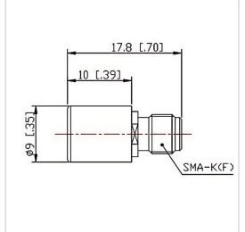
RF Solution offer a wide selection of Coaxial Fixed Termination (Dummy Load) for global customers. CT-02W-RA0910-SK-4G is a Coaxial Fixed Termination (Dummy Load) in Frequency Range of DC~4.0 GHz. It is made of high quality materials under a high standard, the Connector Type of this product is SMA-F (K), VSWR Max is 1.20 and Impedance is 50  $\Omega$ . The component has a good working performance and stability, it is ideal for handling a Power of 2 W.
