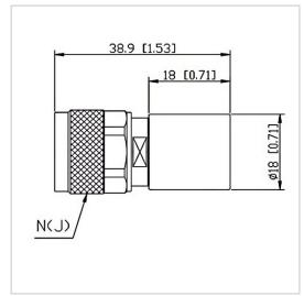
RF Solution offer a wide selection of Coaxial Fixed Termination (Dummy Load) for global customers. CT-02W-RA1818-NJ-18G is Coaxial Fixed а Termination (Dummy Load) in Frequency Range of DC~18.0 GHz. It is made of high quality materials under a high standard, the Connector Type of this product is N-M (J), VSWR Max is 1.25 and Impedance is 50  $\Omega$ . The component has a good working performance and stability, it is ideal for handling a Power of 2 W.
