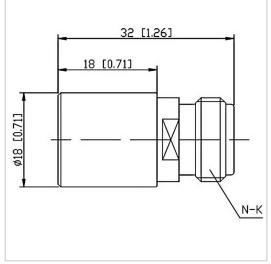
RF Solution offer a wide selection of Coaxial Fixed Termination (Dummy Load) for global customers. CT-02W-RA1818-NK-10G is Coaxial Fixed Termination (Dummy Load) in Frequency Range of DC~10.0 GHz. It is made of high quality materials under a high standard, the Connector Type of this product is N-F (K), VSWR Max is 1.25 and Impedance is 50  $\Omega$ . The component has a good working performance and stability, it is ideal for handling a Power of 2 W.
