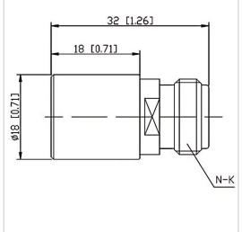
RF Solution offer a wide selection of Coaxial Fixed Termination (Dummy Load) for global customers. CT-02W-RA1818-NK-12.4G is Coaxial Termination (Dummy Load) in Frequency Range of DC~12.4 GHz. It is made of high quality materials under a high standard, the Connector Type of this product is N-F (K), VSWR Max is 1.25 and Impedance is 50  $\Omega$ . The component has a good working performance and stability, it is ideal for handling a Power of 2 W.
