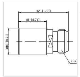
RF Solution offer a wide selection of Coaxial Fixed Termination (Dummy Load) for global customers. CT-02W-RA1818-NK-8G is a Coaxial Fixed Termination (Dummy Load) in Frequency Range of DC~8.0 GHz. It is made of high quality materials under a high standard, the Connector Type of this product is N-F (K), VSWR Max is 1.20 and Impedance is 50  $\Omega$ . The component has a good working performance and stability, it is ideal for handling a Power of 2 W.
