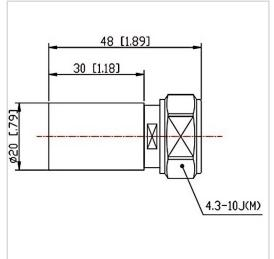
RF Solution offer a wide selection of Coaxial Fixed Termination (Dummy Load) for global customers. CT-02W-RA2030-4310J-4G is a Coaxial Fixed Termination (Dummy Load) in Frequency Range of DC~4.0 GHz. It is made of high quality materials under a high standard, the Connector Type of this product is 4.3-10-M (J), VSWR Max is 1.20 and Impedance is 50  $\Omega$ . The component has a good working performance and stability, it is ideal for handling a Power of 2 W.
