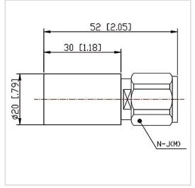
RF Solution offer a wide selection of Coaxial Fixed Termination (Dummy Load) for global customers. CT-02W-RA2030-NJ-6G is a Coaxial Fixed Termination (Dummy Load) in Frequency Range of DC~6.0 GHz. It is made of high quality materials under a high standard, the Connector Type of this product is N-M (J), VSWR Max is 1.25 and Impedance is 50  $\Omega$ . The component has a good working performance and stability, it is ideal for handling a Power of 2 W.
