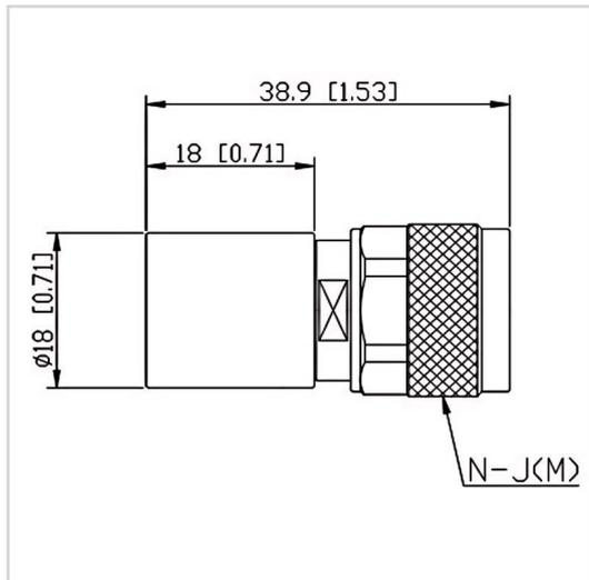
RF Solution offer a wide selection of Coaxial Fixed Termination (Dummy Load) for global customers. CT-05W-RA1818-NJ-10G is a Coaxial Fixed Termination (Dummy Load) in Frequency Range of DC~10.0 GHz. It is made of high quality materials under a high standard, the Connector Type of this product is N-M (J), VSWR Max is 1.25 and Impedance is 50 Ω. The component has a good working performance and stability, it is ideal for handling a Power of 5 W.
