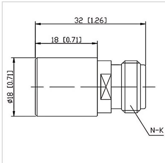
RF Solution offer a wide selection of Coaxial Fixed Termination (Dummy Load) for global customers. CT-05W-RA1818-NK-8G is a Coaxial Fixed Termination (Dummy Load) in Frequency Range of DC~8.0 GHz. It is made of high quality materials under a high standard, the Connector Type of this product is N-F (K), VSWR Max is 1.20 and Impedance is 50 Ω. The component has a good working performance and stability, it is ideal for handling a Power of 5 W.
