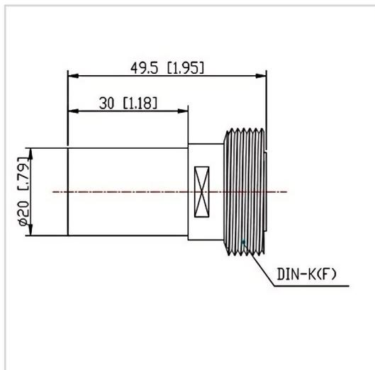
RF Solution offer a wide selection of Coaxial Fixed Termination (Dummy Load) for global customers. CT-05W-RA2030-DINK-4G is a Coaxial Fixed Termination (Dummy Load) in Frequency Range of DC~4.0 GHz. It is made of high quality materials under a high standard, the Connector Type of this product is DIN-F (K), VSWR Max is 1.25 and Impedance is 50  $\Omega$ . The component has a good working performance and stability, it is ideal for handling a Power of 5 W.
