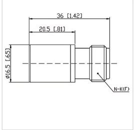
RF Solution offer a wide selection of Coaxial Fixed Termination (Dummy Load) for global customers. CT-05W-RF1620-NK-3G is a Coaxial Fixed Termination (Dummy Load) in Frequency Range of DC $\sim$ 3.0 GHz. It is made of high quality materials under a high standard, the Connector Type of this product is N-F (K), VSWR Max is 1.20 and Impedance is 50  $\Omega$ . The component has a good working performance and stability, it is ideal for handling a Power of 5 W.
