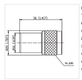
RF Solution offer a wide selection of Coaxial Fixed Termination (Dummy Load) for global customers. CT-05W-RF2036-NJ-3G is a Coaxial Fixed Termination (Dummy Load) in Frequency Range of DC $\sim$ 3.0 GHz. It is made of high quality materials under a high standard, the Connector Type of this product is N-M (J), VSWR Max is 1.20 and Impedance is 50  $\Omega$ . The component has a good working performance and stability, it is ideal for handling a Power of 5 W.
