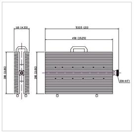
RF Solution offer a wide selection of Coaxial Fixed Termination (Dummy Load) for global customers. CT-1000W-FF3049-DINK-1G is a Coaxial Fixed Termination (Dummy Load) in Frequency Range of DC~1.0 GHz. It is made of high quality materials under a high standard, the Connector Type of this product is DIN-F (K), VSWR Max is 1.35 and Impedance is 50  $\Omega$ . The component has a good working performance and stability, it is ideal for handling a Power of 1000 W.
