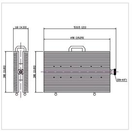
RF Solution offer a wide selection of Coaxial Fixed Termination (Dummy Load) for global customers. CT-1000W-FF3049-DINK-2G is a Coaxial Fixed Termination (Dummy Load) in Frequency Range of DC~2.0 GHz. It is made of high quality materials under a high standard, the Connector Type of this product is DIN-F (K), VSWR Max is 1.35 and Impedance is 50  $\Omega$ . The component has a good working performance and stability, it is ideal for handling a Power of 1000 W.
