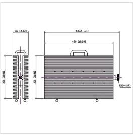
RF Solution offer a wide selection of Coaxial Fixed Termination (Dummy Load) for global customers. CT-1000W-FF3049-DINK-3G is a Coaxial Fixed Termination (Dummy Load) in Frequency Range of DC $\sim$ 3.0 GHz. It is made of high quality materials under a high standard, the Connector Type of this product is DIN-F (K), VSWR Max is 1.35 and Impedance is 50  $\Omega$ . The component has a good working performance and stability, it is ideal for handling a Power of 1000 W.
