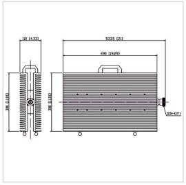
RF Solution offer a wide selection of Coaxial Fixed Termination (Dummy Load) for global customers. CT-1000W-FF3049-DINK-4G is a Coaxial Fixed Termination (Dummy Load) in Frequency Range of DC~4.0 GHz. It is made of high quality materials under a high standard, the Connector Type of this product is DIN-F (K), VSWR Max is 1.35 and Impedance is 50  $\Omega$ . The component has a good working performance and stability, it is ideal for handling a Power of 1000 W.
