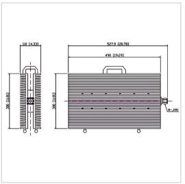
RF Solution offer a wide selection of Coaxial Fixed Termination (Dummy Load) for global customers. CT-1000W-FF3049-NJ-1G is a Coaxial Fixed Termination (Dummy Load) in Frequency Range of DC $\sim$ 1.0 GHz. It is made of high quality materials under a high standard, the Connector Type of this product is N-M (J), VSWR Max is 1.35 and Impedance is 50  $\Omega$ . The component has a good working performance and stability, it is ideal for handling a Power of 1000 W.
