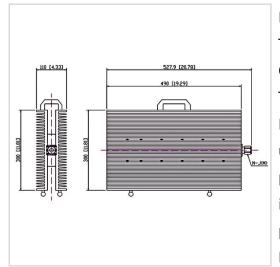
RF Solution offer a wide selection of Coaxial Fixed Termination (Dummy Load) for global customers. CT-1000W-FF3049-NJ-2G is a Coaxial Fixed Termination (Dummy Load) in Frequency Range of DC~2.0 GHz. It is made of high quality materials under a high standard, the Connector Type of this product is N-M (J), VSWR Max is 1.35 and Impedance is 50  $\Omega$ . The component has a good working performance and stability, it is ideal for handling a Power of 1000 W.
