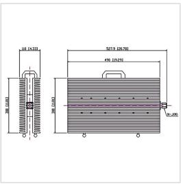
RF Solution offer a wide selection of Coaxial Fixed Termination (Dummy Load) for global customers. CT-1000W-FF3049-NJ-3G is a Coaxial Fixed Termination (Dummy Load) in Frequency Range of DC $\sim$ 3.0 GHz. It is made of high quality materials under a high standard, the Connector Type of this product is N-M (J), VSWR Max is 1.35 and Impedance is 50  $\Omega$ . The component has a good working performance and stability, it is ideal for handling a Power of 1000 W.
