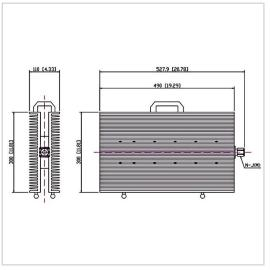
RF Solution offer a wide selection of Coaxial Fixed Termination (Dummy Load) for global customers. CT-1000W-FF3049-NJ-4G is a Coaxial Fixed Termination (Dummy Load) in Frequency Range of DC~4.0 GHz. It is made of high quality materials under a high standard, the Connector Type of this product is N-M (J), VSWR Max is 1.45 and Impedance is 50  $\Omega$ . The component has a good working performance and stability, it is ideal for handling a Power of 1000 W.
