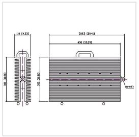
RF Solution offer a wide selection of Coaxial Fixed Termination (Dummy Load) for global customers. CT-1000W-FF3049-NK-2G is Coaxial Termination (Dummy Load) in Frequency Range of DC~2.0 GHz. It is made of high quality materials under a high standard, the Connector Type of this product is N-F (K), VSWR Max is 1.35 and Impedance is 50  $\Omega$ . The component has a good working performance and stability, it is ideal for handling a Power of 1000 W.
