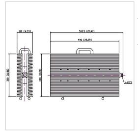
RF Solution offer a wide selection of Coaxial Fixed Termination (Dummy Load) for global customers. CT-1000W-FF3049-NK-3G is a Coaxial Fixed Termination (Dummy Load) in Frequency Range of DC~3.0 GHz. It is made of high quality materials under a high standard, the Connector Type of this product is N-F (K), VSWR Max is 1.35 and Impedance is 50  $\Omega$ . The component has a good working performance and stability, it is ideal for handling a Power of 1000 W.
