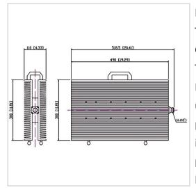
RF Solution offer a wide selection of Coaxial Fixed Termination (Dummy Load) for global customers. CT-1000W-FF3049-NK-4G is a Coaxial Fixed Termination (Dummy Load) in Frequency Range of DC~4.0 GHz. It is made of high quality materials under a high standard, the Connector Type of this product is N-F (K), VSWR Max is 1.45 and Impedance is 50  $\Omega$ . The component has a good working performance and stability, it is ideal for handling a Power of 1000 W.
