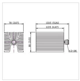
RF Solution offer a wide selection of Coaxial Fixed Termination (Dummy Load) for global customers. CT-100W-FA8011-4310K-6G is a Coaxial Fixed Termination (Dummy Load) in Frequency Range of DC $\sim$ 6.0 GHz. It is made of high quality materials under a high standard, the Connector Type of this product is 4.3-10-F (K), VSWR Max is 1.30 and Impedance is 50  $\Omega$ . The component has a good working performance and stability, it is ideal for handling a Power of 100 W.
