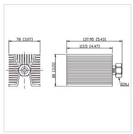
RF Solution offer a wide selection of Coaxial Fixed Termination (Dummy Load) for global customers. CT-100W-FA8011-DINJ-3G is a Coaxial Fixed Termination (Dummy Load) in Frequency Range of DC $\sim$ 3.0 GHz. It is made of high quality materials under a high standard, the Connector Type of this product is DIN-M (J), VSWR Max is 1.20 and Impedance is 50  $\Omega$ . The component has a good working performance and stability, it is ideal for handling a Power of 100 W.
