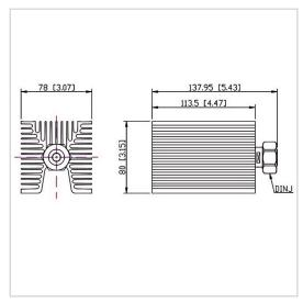
RF Solution offer a wide selection of Coaxial Fixed Termination (Dummy Load) for global customers. CT-100W-FA8011-DINJ-4G is a Coaxial Fixed Termination (Dummy Load) in Frequency Range of DC~4.0 GHz. It is made of high quality materials under a high standard, the Connector Type of this product is DIN-M (J), VSWR Max is 1.30 and Impedance is 50  $\Omega$ . The component has a good working performance and stability, it is ideal for handling a Power of 100 W.
