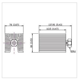
RF Solution offer a wide selection of Coaxial Fixed Termination (Dummy Load) for global customers. CT-100W-FA8011-DINJ-6G is a Coaxial Fixed Termination (Dummy Load) in Frequency Range of DC~6.0 GHz. It is made of high quality materials under a high standard, the Connector Type of this product is DIN-M (J), VSWR Max is 1.30 and Impedance is 50  $\Omega$ . The component has a good working performance and stability, it is ideal for handling a Power of 100 W.
