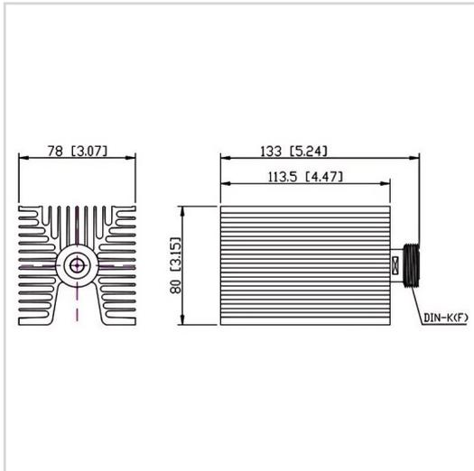
RF Solution offer a wide selection of Coaxial Fixed Termination (Dummy Load) for global customers. CT-100W-FA8011-DINK-4G is a Coaxial Fixed Termination (Dummy Load) in Frequency Range of DC~4.0 GHz. It is made of high quality materials under a high standard, the Connector Type of this product is DIN-F (K), VSWR Max is 1.30 and Impedance is 50  $\Omega$ . The component has a good working performance and stability, it is ideal for handling a Power of 100 W.
