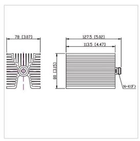
RF Solution offer a wide selection of Coaxial Fixed Termination (Dummy Load) for global customers. CT-100W-FA8011-NK-4G is Coaxial Termination (Dummy Load) in Frequency Range of DC~4.0 GHz. It is made of high quality materials under a high standard, the Connector Type of this product is N-F (K), VSWR Max is 1.25 and Impedance is 50  $\Omega$ . The component has a good working performance and stability, it is ideal for handling a Power of 100 W.
