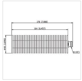
RF Solution offer a wide selection of Coaxial Fixed Termination (Dummy Load) for global customers. CT-100W-RA4816-NK-10G is a Coaxial Fixed Termination (Dummy Load) in Frequency Range of DC~10.0 GHz. It is made of high quality materials under a high standard, the Connector Type of this product is N-F (K), VSWR Max is 1.30 and Impedance is 50  $\Omega$ . The component has a good working performance and stability, it is ideal for handling a Power of 100 W.
