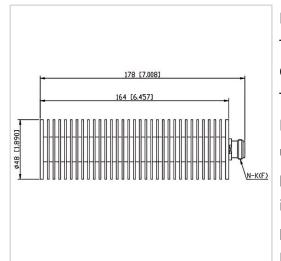
RF Solution offer a wide selection of Coaxial Fixed Termination (Dummy Load) for global customers. CT-100W-RA4816-NK-12.4G is a Coaxial Fixed Termination (Dummy Load) in Frequency Range of DC~12.4 GHz. It is made of high quality materials under a high standard, the Connector Type of this product is N-F (K), VSWR Max is 1.35 and Impedance is 50  $\Omega$ . The component has a good working performance and stability, it is ideal for handling a Power of 100 W.
