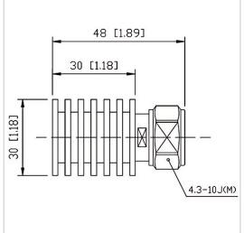
RF Solution offer a wide selection of Coaxial Fixed Termination (Dummy Load) for global customers. CT-10W-RA3030-4310J-3G is а Coaxial Termination (Dummy Load) in Frequency Range of DC~3.0 GHz. It is made of high quality materials under a high standard, the Connector Type of this product is 4.3-10-M (J), VSWR Max is 1.20 and Impedance is 50  $\Omega$ . The component has a good working performance and stability, it is ideal for handling a Power of 10 W.
