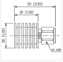
RF Solution offer a wide selection of Coaxial Fixed Termination (Dummy Load) for global customers. CT-10W-RA3030-NJ-4G is a Coaxial Fixed Termination (Dummy Load) in Frequency Range of DC $\sim$ 4.0 GHz. It is made of high quality materials under a high standard, the Connector Type of this product is N-M (J), VSWR Max is 1.20 and Impedance is 50  $\Omega$ . The component has a good working performance and stability, it is ideal for handling a Power of 10 W.
