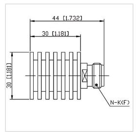
RF Solution offer a wide selection of Coaxial Fixed Termination (Dummy Load) for global customers. CT-10W-RA3030-NK-4G is a Coaxial Fixed Termination (Dummy Load) in Frequency Range of DC~4.0 GHz. It is made of high quality materials under a high standard, the Connector Type of this product is N-F (K), VSWR Max is 1.20 and Impedance is 50  $\Omega$ . The component has a good working performance and stability, it is ideal for handling a Power of 10 W.
