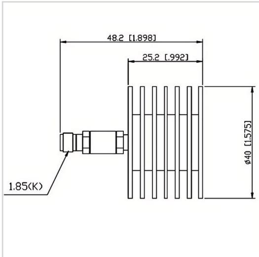
RF Solution offer a wide selection of Coaxial Fixed Termination (Dummy Load) for global customers. CT-10W-RA4025-1.85K-67G is a Coaxial Fixed Termination (Dummy Load) in Frequency Range of DC~67.0 GHz. It is made of high quality materials under a high standard, the Connector Type of this product is 1.85-F (K), VSWR Max is 1.40 and Impedance is 50 Ω. The component has a good working performance and stability, it is ideal for handling a Power of 10 W.
