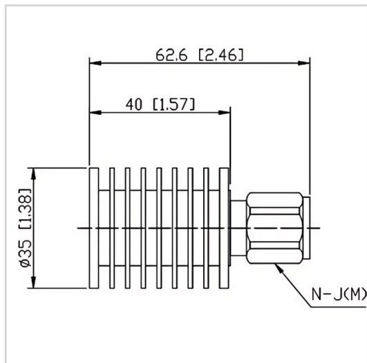
RF Solution offer a wide selection of Coaxial Low PIM Termination for global customers. CT-10W-RH3540-IP65-NJ-3G is a Coaxial Low PIM Termination in Frequency Range of DC~3.0 GHz. It is made of high quality materials under a high standard, the Connector Type of this product is N-M (J), VSWR Max is 1.20 and Impedance is 50 Ω. The component has a good working performance and stability, it is ideal for handling a Power of 10 W.
