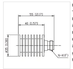
RF Solution offer a wide selection of Coaxial Low PIM Termination for global customers. CT-10W-RH3540-IP65-NK-3G is a Coaxial Low PIM Termination in Frequency Range of DC~3.0 GHz. It is made of high quality materials under a high standard, the Connector Type of this product is N-F (K), VSWR Max is 1.20 and Impedance is 50  $\Omega$ . The component has a good working performance and stability, it is ideal for handling a Power of 10 W.
