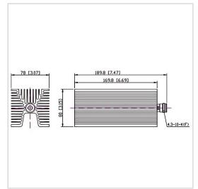
RF Solution offer a wide selection of Coaxial Fixed Termination (Dummy Load) for global customers. CT-150W-FA8017-4310K-4G is a Coaxial Fixed Termination (Dummy Load) in Frequency Range of DC~4.0 GHz. It is made of high quality materials under a high standard, the Connector Type of this product is 4.3-10-F (K), VSWR Max is 1.30 and Impedance is 50  $\Omega$ . The component has a good working performance and stability, it is ideal for handling a Power of 150 W.
