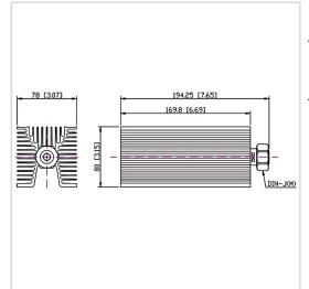
RF Solution offer a wide selection of Coaxial Fixed Termination (Dummy Load) for global customers. CT-150W-FA8017-DINJ-3G is a Coaxial Fixed Termination (Dummy Load) in Frequency Range of DC~3.0 GHz. It is made of high quality materials under a high standard, the Connector Type of this product is DIN-M (J), VSWR Max is 1.25 and Impedance is 50  $\Omega$ . The component has a good working performance and stability, it is ideal for handling a Power of 150 W.
