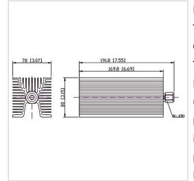
RF Solution offer a wide selection of Coaxial Fixed Termination (Dummy Load) for global customers. CT-150W-FA8017-NJ-4G is a Coaxial Fixed Termination (Dummy Load) in Frequency Range of DC~4.0 GHz. It is made of high quality materials under a high standard, the Connector Type of this product is N-M (J), VSWR Max is 1.25 and Impedance is 50  $\Omega$ . The component has a good working performance and stability, it is ideal for handling a Power of 150 W.
