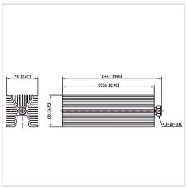
RF Solution offer a wide selection of Coaxial Fixed Termination (Dummy Load) for global customers. CT-200W-FA8022-4310J-3G is a Coaxial Termination (Dummy Load) in Frequency Range of DC~3.0 GHz. It is made of high quality materials under a high standard, the Connector Type of this product is 4.3-10-M (J), VSWR Max is 1.25 and Impedance is 50  $\Omega$ . The component has a good working performance and stability, it is ideal for handling a Power of 200 W.
