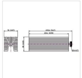
RF Solution offer a wide selection of Coaxial Fixed Termination (Dummy Load) for global customers. CT-200W-FA8022-DINK-6G is a Coaxial Fixed Termination (Dummy Load) in Frequency Range of DC~6.0 GHz. It is made of high quality materials under a high standard, the Connector Type of this product is DIN-F (K), VSWR Max is 1.30 and Impedance is 50  $\Omega$ . The component has a good working performance and stability, it is ideal for handling a Power of 200 W.
